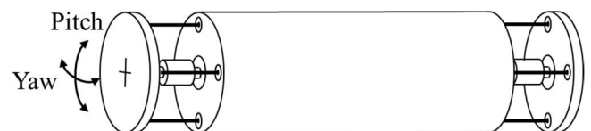
Figure 22. Actuation in pitch and yaw rotational direction at left and right end of the robot arm segment.
