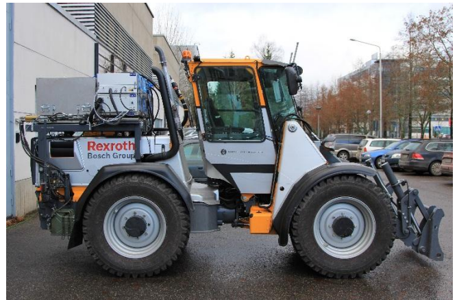
Figure 1: Wille-municipal tractor with the portable emission measurement system.
