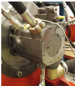
Figure 1: Bosch A11VO pump studied in the paper.
